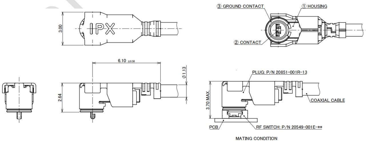
Figure : Space Factor of Mated Connectors (Unit:mm)
